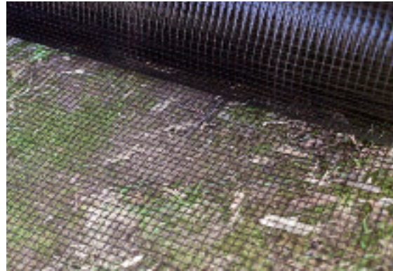
You can identify the MAX Strength layer by looking at the size of the opening. It is one inch and it is metal.
